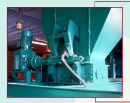
We produce the shredders on the CNC-machines. The output inspection secures the quality of individual components. The stand and feeding hopper are construed with regard to securing the safety of the atten-dance and the size of the output of the equipment, which a container can be directly.
